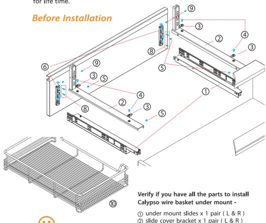
NJA8601 is designed for 450 mm deep basket. Recommended screw for *slide mounting* – #8 round head screw
