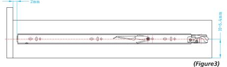
Fix the drawer member through vertical slots for vertical adjustment. Leave the screw loose for final adjustment.
