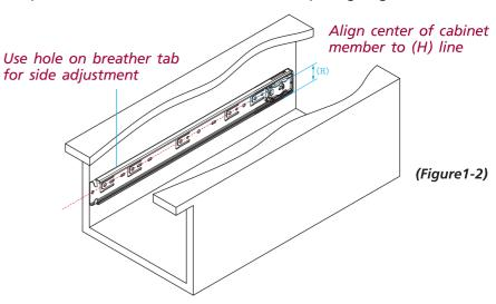
Fix the slides through the most flexible holes on breather tab for best slide performance. Leave the screw loose for final adjustment. Move the slides back and forth, and make sure no screw is bound.
