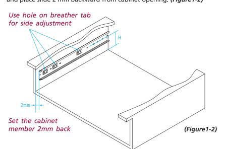
Fix the slides through the most flexible holes on breather tab for best slide performance. Leave the screw loose for final adjustment. Move the slides back and forth, and make sure no screw is bound.
