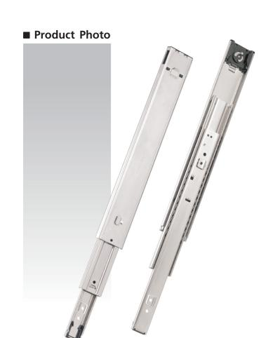
**Features ■** Profile Mounting | Side mount. Slide Clearance | 18.0 mm plus 1/64", minus 0 each Height | 57.4 mm **■** Surface Treatment Loading | 160 pound (72 kgs) class. ■ Clear Zinc ■ Black Zinc **Size** | 419.10 mm ■ Black E. Coating ■ White E Coating Feature | Bayonet mount, rear interlock. ■ Galvanized Steel Option | None. ■ Stainless Steel ■ Packaging
