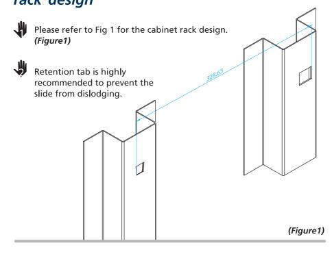
For the ease of installation, suggest mounting the slides from the bottom to the top.
