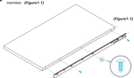
Align the center line of drawer member to the center line of keyboard shelf. (Figure 1-2) LIFT UP OR
