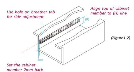
Fix the slides through the most flexible holes on breather tab for best slide performance. Leave the screw loose for final adjustment. Move the slides back and forth, and make sure no screw is bound.
