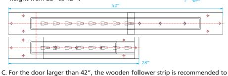
assure the smooth operation, and the 3rd slide is suggested to be utilized for a better load capacity.
