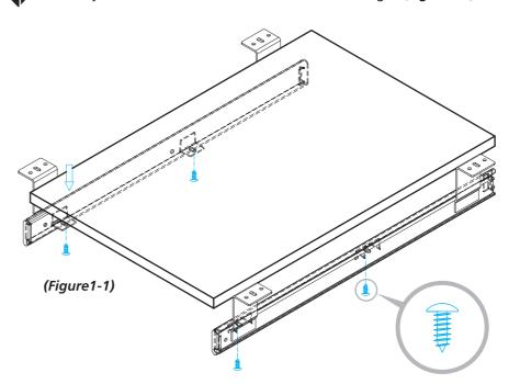
Screw the shelf through the slot on shelf tab from the bottom. (Figure 1-2)
