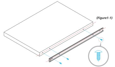
Align the center line of drawer member to the center line of keyboard
