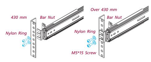
B. Attach the L-shaped bracket to the rear mounting flange using M5\*12 screw & 12 mm nylon ring from screw kit, then tighten rear bracket mounting
