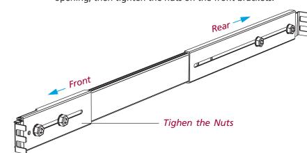
**Step 3>** Extend the rear brackets to where it reaches the rear rack. Do not fully tighten rear bracket mounting screws until final adjustment is made.
