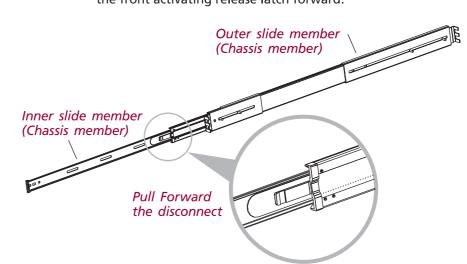
Step 2> Each slide is pre-attached with front (W-528) and rear (W-529) adjustable EIA brackets. Loosen the nuts on the both brackets, and decide the proper setback distance to the opening, then tighten the nuts on the front brackets.
