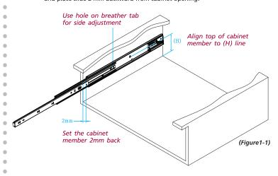
Fix the slides through the countersunk holes, and leave the screw loose for final adjustment. Move the slides back and forth, and make sure no screw is bound.
