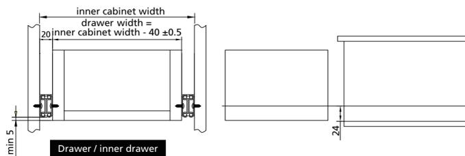
The bottom of drawer slides must be 5mm above the bottom of drawer to ensure correct function. The center of drawer slides must be 24mm above the bottom of cabinet.
